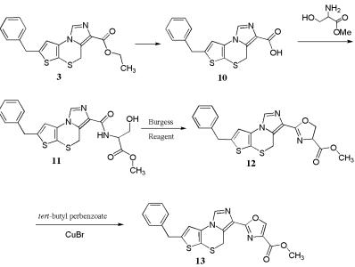
Therefore ethylester **3** was hydrolized with 5% aqueous sodiumhydroxide to give compound **10**. Reaction with D,L-serine methyl ester gave intermediate **11** which was cyclized by adding Burgess Reagent to yield **12** [10]. Finally dehydrogenation of **12** was carried out with *tert*-butyl perbenzoate and copper-(I)-bromide following the reaction of Kharasch-Sosnovsky to get the desired product **13** [11].
